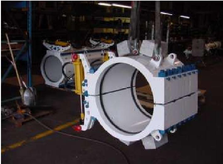
48" Sub-sea Clamp ANSI Class 600 – 4ft long Oil line – with hydraulic activation and sub-sea anodes located at Nigeria
