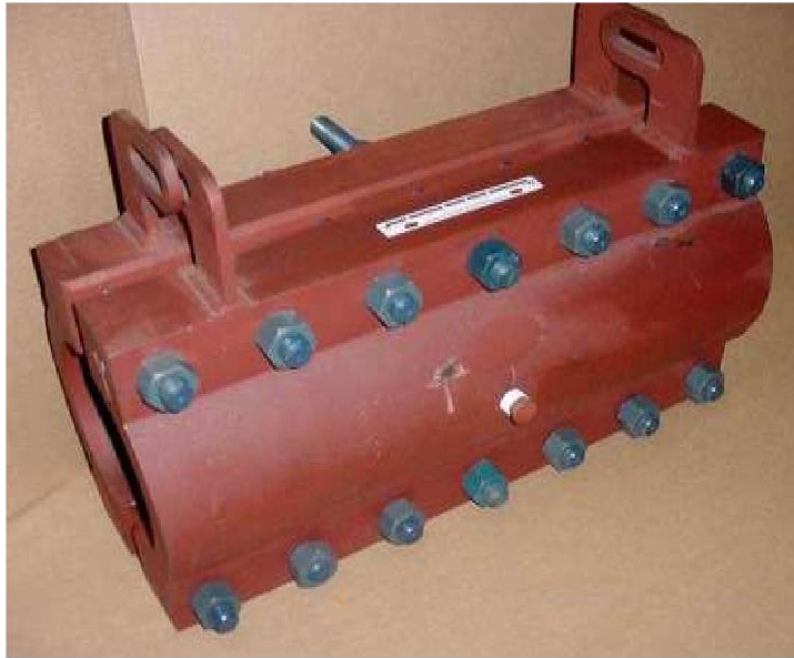
SSRC- Extra Long 6 Inch Nom. 24 Inch Seal Length 1500 PSI MAOP
