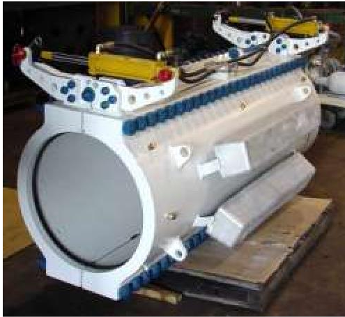
24 Inch Nom. X 88 Inch Subsea SSRC With Hydraulic Controls
