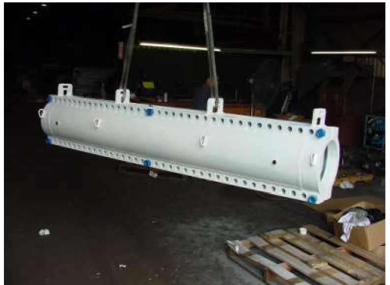
12" ANSI Class 600 – Sub-sea clamp – 10ft long for gas line repair - located at Gulf of Mexico
